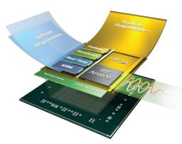
The AMD Zynq® UltraScale+™ RFSoC integrates RF-class A/D and D/A converters into the Zynq® FPGA fabric and multi-core ARM processor subsystem, creating a multi-channel data conversion and processing solution on a single chip.
